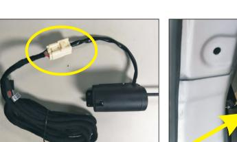
25. As shown in the figure, the socket of the electric suction lock is inserted into our electric suction Hall line socket.
