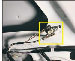
. Locate the grounding screw at the tailgate. Connect the screw to our power ground.
