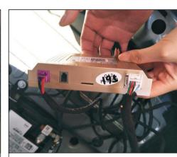
29. Control box white socket, OBD socket and power socket
