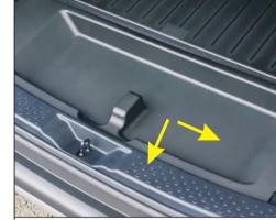
22. Take out the load plate at the tailgate, remove the plaque, and find the original car lock.
