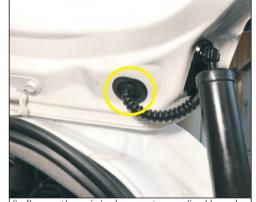
6. Remove the original car waterproof rubber plug on the right side of the car, and the right strut wire passes through the original car rubber plug hole to the tailgate cover.
