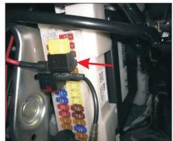
14. Find the original car power under the steering wheel of the main driver, unplug the original car and plug it into our power socket.
