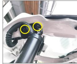
2. Remove the left upper bracket of the original car and install the left upper bracket of our company. The ball head is facing the tailgate and fixed with our screws.
