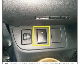
10. Remove the original car empty button at the main driving steering wheel as shown in the figure, and install the front switch button of our company.
