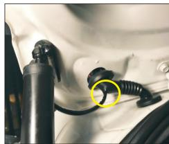
7. Remove the original car waterproof rubber plug on the left side of the car, cut a small hole, and the left strut line passes through the waterproof rubber plug.
