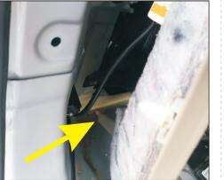
26. The motor is installed on the left side of the tailgate and fixed with our
