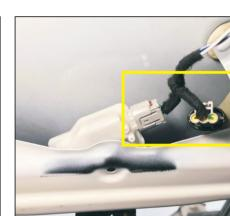
20. Find this terminal housing at the 21. Locate the terminal housing at the tailgate lock and insert the three-way back door and plug it into our front switch adapter socket. adapter socket.
