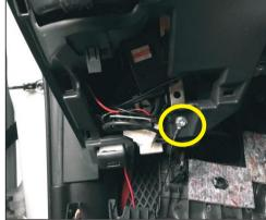
13. The front switch ground wire is connected to the grounding screw below the main steering wheel.
