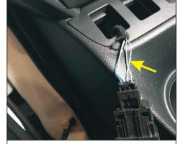
12. The front switch ILL cable is connected to the white green cable of the original car small lamp terminal bousing
