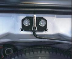
24. Remove the original car lock, install our electric shock lock, and fix it with
