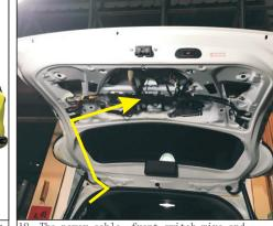
h 18. The power cable, front switch wire and central control wire pass through the waterproof rubber plug along the yellow arrowto the tailgate cover.
