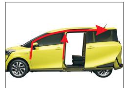
17. The main driving power cable, front switch cable and central control cable are routed from the top of the vehicle body along the red arrow to the tailgate cover.
