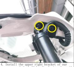
4. Install the upper right bracket of our company, and the ball headis facing the tail door. Use our screws to fix the right upper breaket of the original car.
