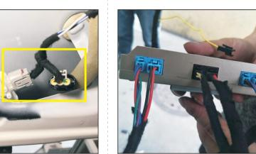
28. The control box plug is inserted according to the color, please check whether the socket is inserted in place.
