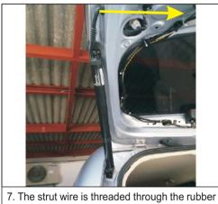
plug hole to the position of the tailgate cover control box
