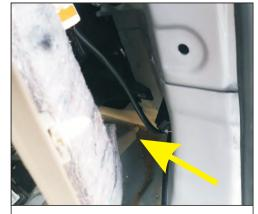
26. The motor is mounted on the right side of the tailgate and fixed with our 3M adhesive.
