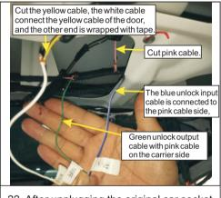
22. After unplugging the original car socket, as shown in the wiring
