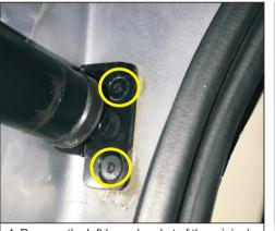
car, install the left lower bracket of our company, and fix it with our screws
