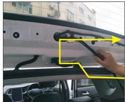
18. The power wire, the front switch wire, and the center wire are routed from the top of the vehicle along the yellow arrow to the tailgate cover
