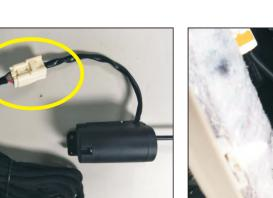
25. As shown in the picture, the electric suction lock socket plugs our electric suction Hall line socket
