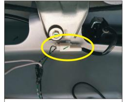
20. Find this terminal housing at the back door and insert the front switch adapter
