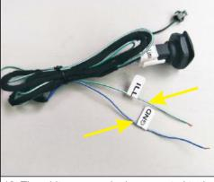
13. The white-green wire is connected to the right side of the steering wheel, punches and | original car light wire by our ILL wire, and the white-blue wire is our ground wire.
