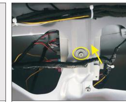
31. Control box installation position, fixed with our screws, gaskets, mesons
