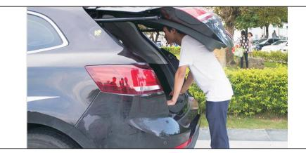
Anti-pinch function: 1. Anti-clamping: When the obstacle is under the tailgate closed, when the tailgate is closed, When you encounter an obstacle, you will bounce back in the opposite direction 2. Door collision avoidance: When the obstacle is behind the tailgate Obstacles will bounce back in the opposite direction
