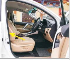
15. Remove the plaque from the main driving seat belt B column
