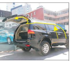
17. The main driving power wire, the front switching wire and the central control wire are routed from the top of the vehicle along the yellow arrow to the tailgate cover
