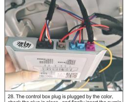
check the plug in place, and finally insert the purple power cord socket
