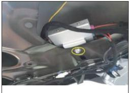
14. Installation position of control box, fixed with our screw, ring and flat washer
