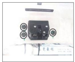
12. Remove the door lock of the original vehicle, install our electric suction lock, and fix it with the screws of the original vehicle.
