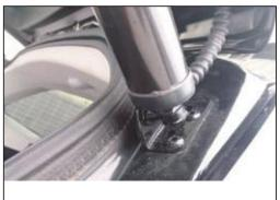
4. Remove the right lower bracket of the original vehicle, install the specially designed lower right bracket, and fix it with the specially designed round head screw (as shown in the figure).
