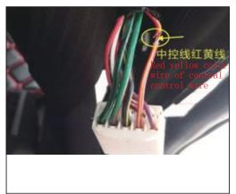
10. Remove the trim board at the B-pillar of the main driver's seat belt and find the central control. Our yellow central control wire connects the red and yellow line of the seat (the fourth hole in the first row from left to right).
