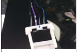
11. Unplug this socket at the original vehicle door lock to plug in the three-way adapter socket
