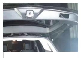
15. Remove the trim board, punch holes in the trim board and install the tailgate switch button.
