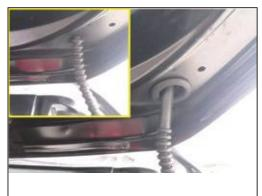
6. As shown in the figure, the hall line passes through the reserved hole and plug in the rubber plug (the same as the left and right steps).
