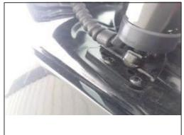
3. Remove the left lower bracket of the original vehicle, install the special left lower bracket, and fix it with the specially designed round head screw.
