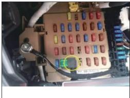
8. Remove the trim board under the main driver, pull out the 15A fuse of the original car and insert our power plug into it.
