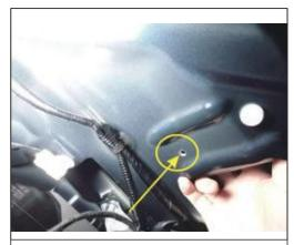
18. Installation position of control box, fixed with company's screw, ring and spring
