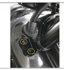
3. Remove the left lower bracket and electric pole of the original car, install the left lower bracket and electric pole of our company
