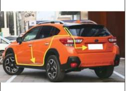
14. The power supply cable and the central control cable run along the car body to the tailgate control box.
