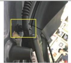
2. Remove the ball head of the original car, install the ball head of our company, add a flat washer underneath to install the electric pole of our company, with the end of the cable socket facing up (the same steps are left and right)
