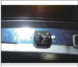
15. Remove the trim board from the trunk and find the original car latch
