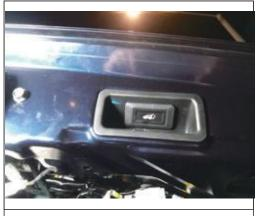
19. Remove the original car trim panel, punch hole and install our company's tailgate switch
