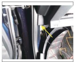
10. Find the grounding screw on the main driver's compartment side
