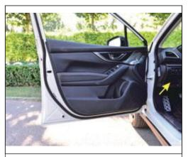
7. Remove the trim board from the main driver compartment and find the power supply
