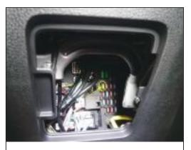
$4.\ Remove$  the plaque found below main driving power supply, unplug the original car yellow 20 a fuse, plug in our power plug
