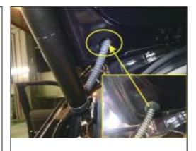
3. Remove the original car waterproof glue plug, wire poles through the original car door hole go line to end control box, card rubber plug
