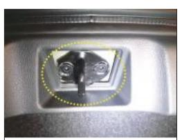
10. Remove the original lock buckle, installing special lock, with screws
