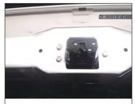
15.Remove the screw of the original car, remove the suction lock of the original car, install our electric suction lock, and fix it with the screw of the original car.
