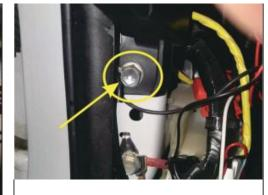
9.Remove the trim board at the side of the driver compartment, loosen the screw and connect the ground wire then tighten the screw.
