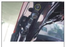
4. Install our electric pole with the upper bracket of the original car (the same steps are left and right)
