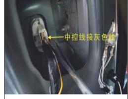
12. The central control wire is connected to grey color wire (the third hole in the second row from left to right)
