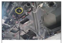
18. Unplug this socket at the tailgate and connect to our front switch socket
