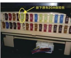
8. Remove the trim board under the driver compartment, pull out the 20A fuse of the original car, and insert our power plug.
