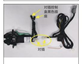
16. As shown in the figure, the socket of the three-way harness is connected to our electric suction socket.
