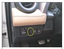
10. At driver compartment takes off the dummy button of the original car and install our front switch button.
