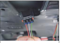
17. Connect the original car unlock plug directly with our provided three-way adapter socket, and plug the other end of our socket to the door lock socket.
