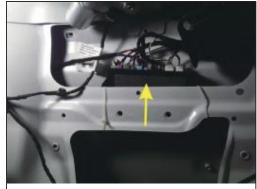
20.Install the control box here, paste our 3M tape on the back of the control box, and secure it with a tie strap.
