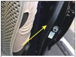
11.At the B-pillar of the driver side seat belt, remove the trim and find the central control wire.
