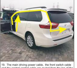
and the central control cable are routed from the top of the vehicle along the yellow arrow to the tailgate cover
