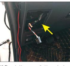
10. The main driver removes the trim panel and can see the original car power supply
