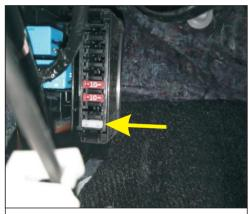
13. The main drive to find the original car power pull the original car 25A fuse
