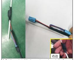
6. Put the socket of the brace wire as shown in the figure, and use the tape to tie the two terminals of the brace to the long brace at the right brace and socket and wrap it tightly with the tape.
