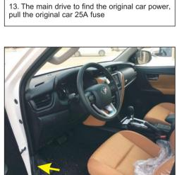
15. The main driver left bottom down remove the plaque to find the grounding screw
