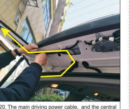
20. The main driving power cable, and the central control cable are routed from the top of the vehicle along the yellow arrow to the tailgate cover
