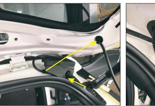
9. The right strut line passes through the rubber stopper of the original vehicle, and goes along the yellow cable to the tailgate cover (same as the left and right steps)
