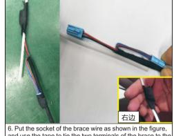
and use the tape to tie the two terminals of the brace to the long brace at the right brace and socket and wrap it tightly
