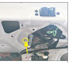
33. Control box installation position, with our screws, gaskets, mesons
