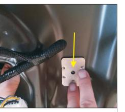
32. Install our control box, add our matching gasket under the panel, and fix it with our screws and gaskets.
