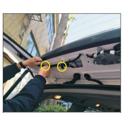
24. Fix the wire harness to the original harness and cut out the extra harness with a pliers.
