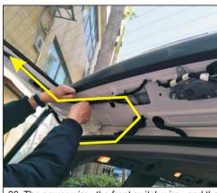
23. The power wire, the front switch wire, and the center wire are routed from the top of the vehicle along the yellow arrow to the tailgate cover
