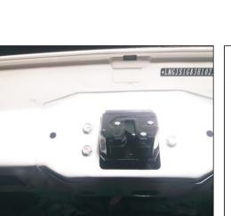
25. Remove the original car screws, remove the original car suction lock, install our electric suction, use the original car screws
