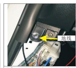
18. Remove the plaque from the lower left side of the co-pilot to find the grounding screw and connect the ground wire.
