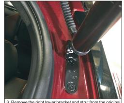
3. Remove the right lower bracket and strut from the original car, install the lower right bracket of our company, engrave with "R", and the arrow faces upwards. The ball head is toward the outside of the body and is fixed with our screws.
