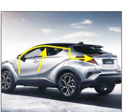
22. The main driving power cable and the central control cable are routed from the top of the vehicle along the yellow arrow to the tailgate cover
