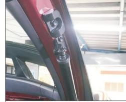
2. Install the company's struts with the right upper bracket of the original car (same as the left and right steps)
