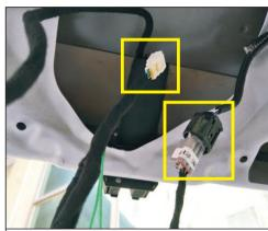
29. Unplug the original car seat at the door lock and insert the three-way adapter socket of our company, and plug the socket of the three-way harness into the electric suction lock
