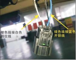
14. At the tail door locks unplug the saddle to take the orange line in the seat of the white line, green line after the blue line
