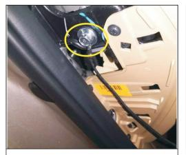
10. In the main drive side remove the plaque, find the ground
