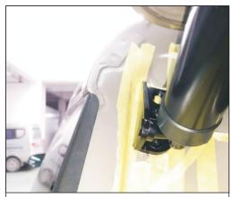
3. Remove the original car bottom bracket, we lower left bracket, installation poles (the line ends of the poles down)
