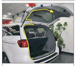
16. Electric door suction line go line 17. Hall line, control line, the power cord to end cove
