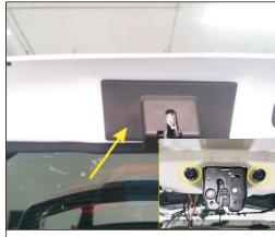
15. Abort the original screw, remove the original car lock, installed on our electric absorption, use the original car screws
