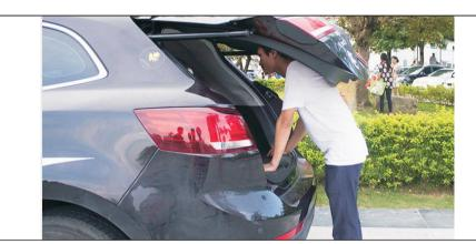
Anti-pinch function: 1. Anti-clamping: When the obstacle is under the tailgate closed, when the tailgate is closed, When you encounter an obstacle, you will bounce back in the opposite direction 2. Door collision avoidance: When the obstacle is behind the tailgate Obstacles will bounce back in the opposite direction
