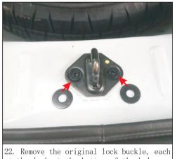
at the lock at the bottom of the hole Add a gasket
