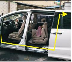
17. The main driving power cord and switch line from the body before walking down the yellow arrow below line to end door cover
