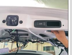
installed special door keys
