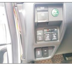
Press the front switch button to open/close the tailgate
