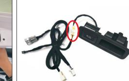
31. Remove the original car trim, 32. The tail door keys with the wire and tee socket to plug socket
