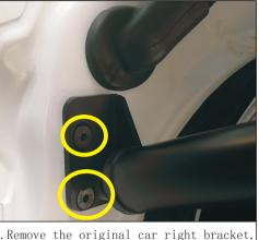
3. Remove the original car right bracket, installation we lower bracket (ball head toward the outside), with our screws
