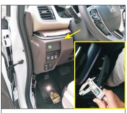
13. Remove the plaque to find the original car white socket
