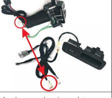
21.As shown on the wire and tee socket to plug our electric socket
