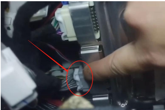
5.拆掉副驾脚窝膝盖处饰板找到行程电脑，电源和协议转接灰色插头 Remove the panel in front the passenger seat to find the trip computer
