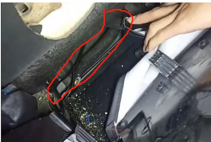
11.走线到座椅后方与上图红框内原车线用扎带绑在一起 Thread the cable to the back of the seat, and bind with the original wire here.
