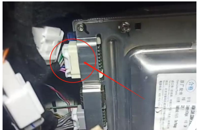
6.音频信号转接上图白色插头 Audio signal cable connect the white plug as the figure shown above.
