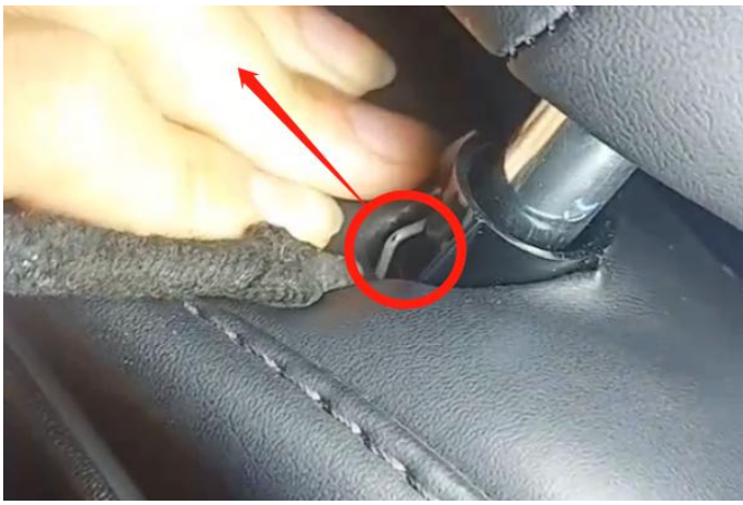
1.把座椅靠垫的上图位置用力往下压，露出里面的卡簧 Press down firmly on the seat cushion at the position shown in the figure above, Expose the snap ring inside.
