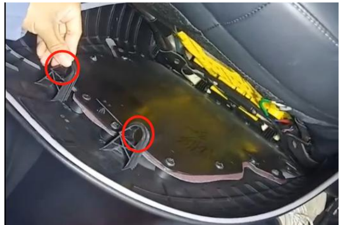
4.座椅靠垫后方盖板主要是上图红圈内两个卡扣固定的 There are two buckle fixed in the seat cushion panel. See the red circle.
