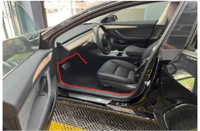
10.头枕线在 ECU 控制盒处穿到马鞍主驾一侧，然后从膝盖饰板内走到门沿橡胶一直到座椅后方（如上图红线示意） Pass through the headrest cable to the another side of the driver's cab, and thread it to the back of the seat.(as the figure shown above.)
